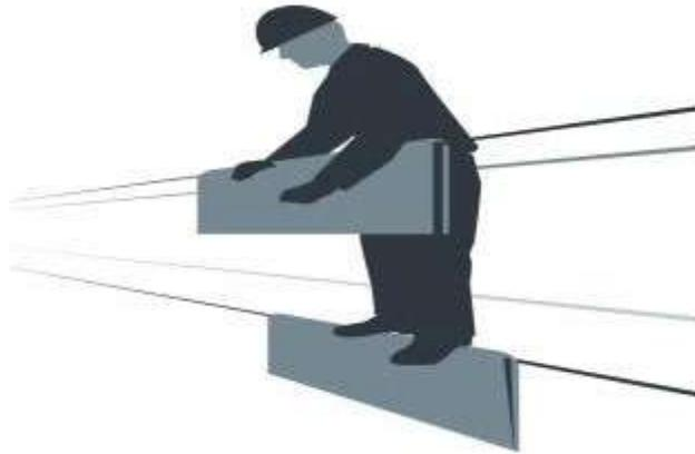
**LV Safety Matting** is mainly used for standing on while working on live switchboards or any other equipment and prevents the possibility of electrocution.
